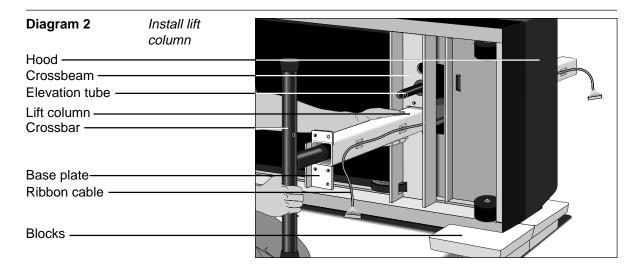
2. Obtain appropriate assistance to lay the treadmill on its left-hand side. Placing the foam blocks on the hood of the treadmill, as shown in Diagram 2, helps elevate the treadmill and keep pressure off the hood and side rail during assembly. Due to the rounded corners on the side rail, one assistant will need to balance the treadmill on its side, while another assistant helps you install the lift column assembly.
